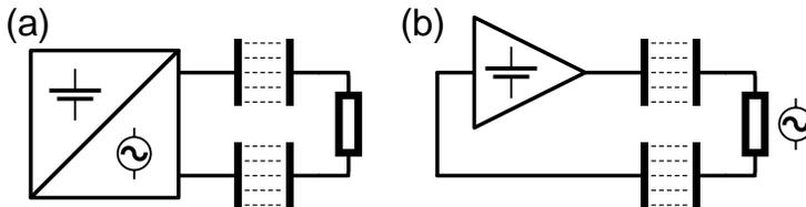
Figure 1: Comparison between the conventional and the proposed WPT systems. (a) In conventional ones, the microwave oscillation is formed in the generator and then transmitted to the load through capacitive wireless link. (b) In the proposed WPT system, the wireless link and the load are part of the feedback loop and the oscillating power is directly generated at the load.
