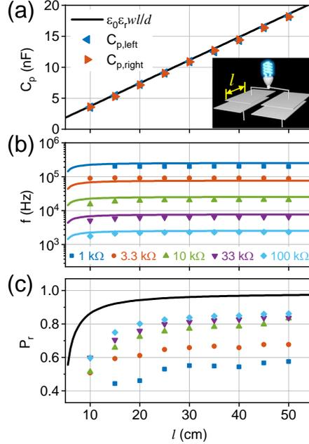
Figure 4: Experimental demonstration of the robustness against receiver position (overlap distance). (a) The plate capacitance is linearly proportional to the overlap distance  $l$  of the aluminum plates. The inset shows how the plates are moved. (b, c) Measured (symbols) and analytic (lines) working frequency and power ratio subjected to the changes of overlap distance. Five load values are measured.
