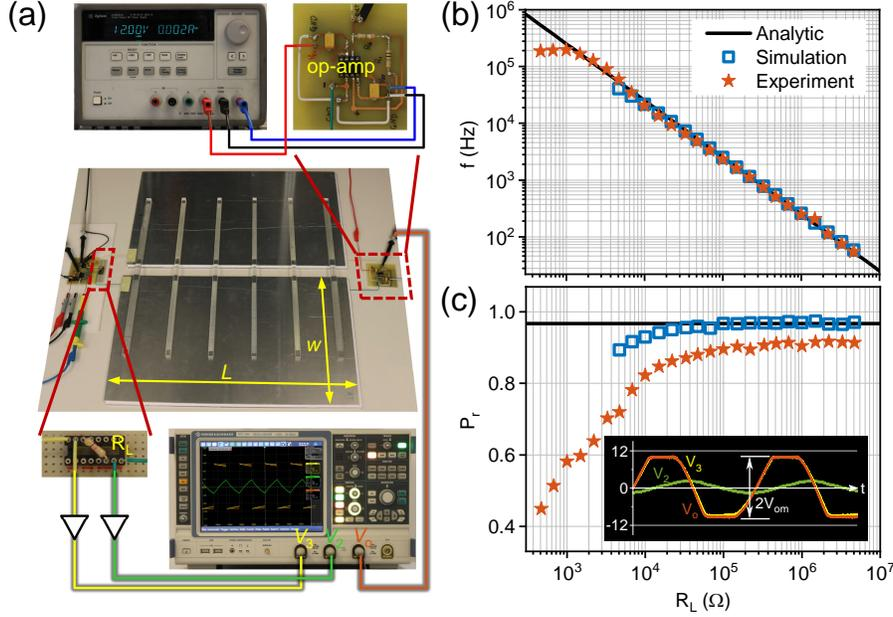
Figure 3: Experimental demonstration of the robustness against load variation. (a) Experimental setup. The capacitive wireless links are made of aluminum plates. (b) Working frequency is inversely proportional to load resistance. (c) Power ratio versus load resistance. The measured value drops when load resistance decreases. The insert shows the experimental voltage oscillations when  $R_L = 1.5 \text{ k}\Omega$ .
