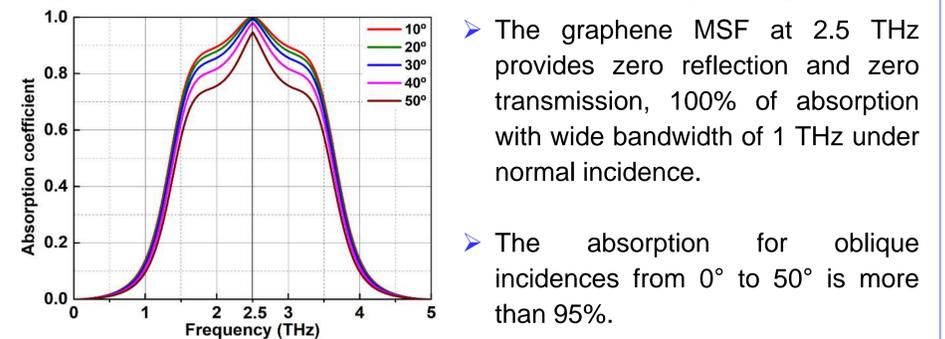
Fig. 6. Absorption spectra of graphene MSF under oblique incidence
