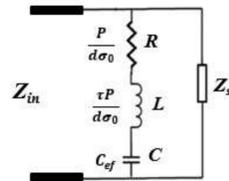
Fig. 4. Equivalent circuit of graphene MSF structure
