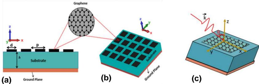
Fig. 3. Schematic of the graphene MSF (a) Cross-sectional view, (b) 3D view, and (c) its unit cell
