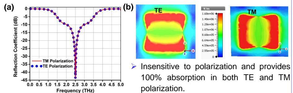
Fig. 7. (a) Reflection spectra and (b) Electric field distribution in TE and TM polarization
