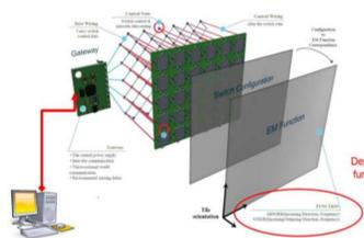
Fig. 1. Architectural overview of Programmable MSF tile
