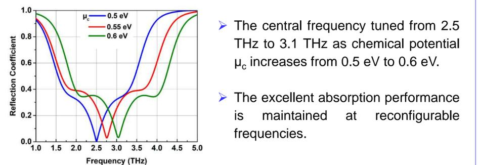
Fig. 8. Frequency reconfiguration of graphene THz MSF surface
