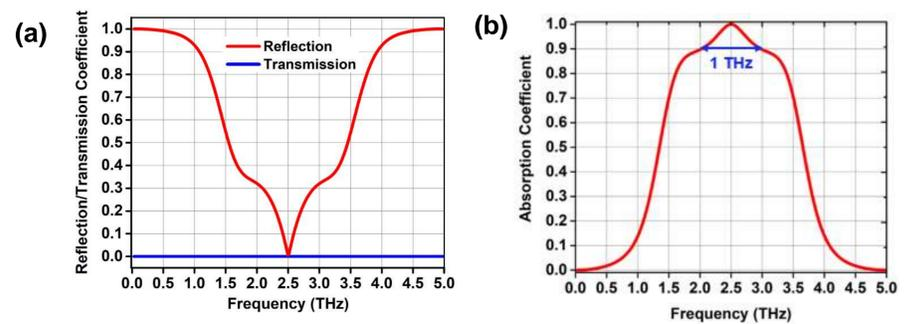
Fig. 5. (a) Reflection and Transmission spectra, and (b) Absorption spectra of graphene MSF
